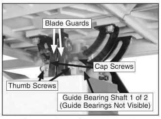
Figure 31. Front of lower blade guide.
